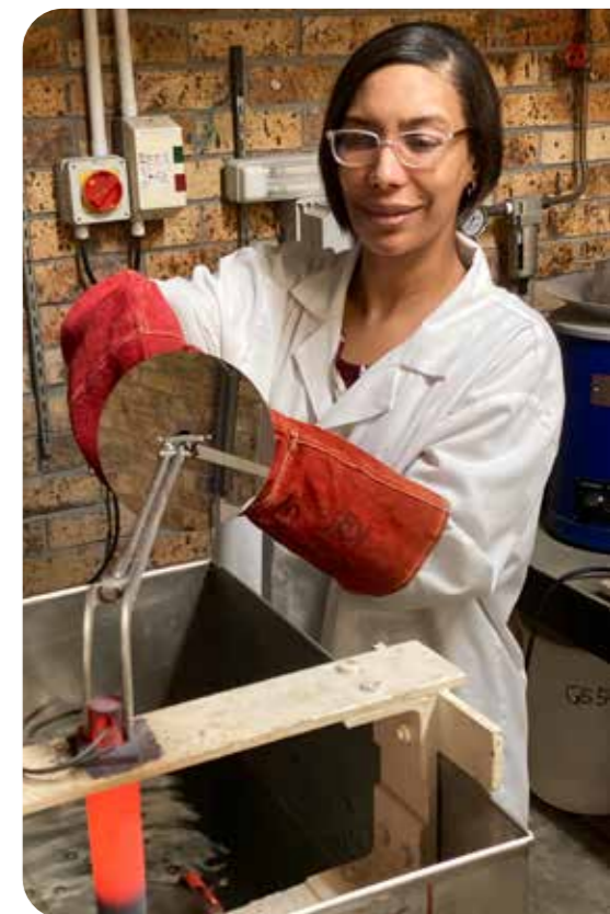
Soraya Allies, PhD researcher in 2021, performing heat treatment simulations of power plant steels in the laboratory
